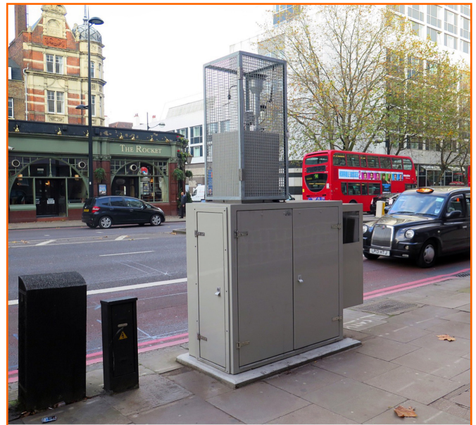
Figure 4. London Air Quality Network (LAQN) roadside monitoring station at Camden - Euston Road Source: London Air (n.d.).
